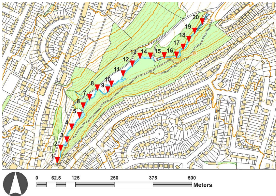
Figure 2: Site locations on the Malago River where water samples were taken and measurements of oxygen saturation, conductivity and pH were made (DigiMap, 2018). In this investigation, site 1 was located at 0m and site 20 was located at 760m downstream.
