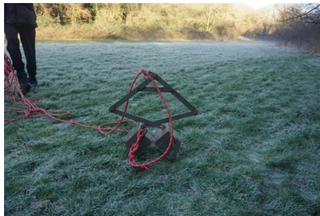
Figure 2. The sediment grabber used for sample collection where channel depth restricted easy access to the riverbed.
